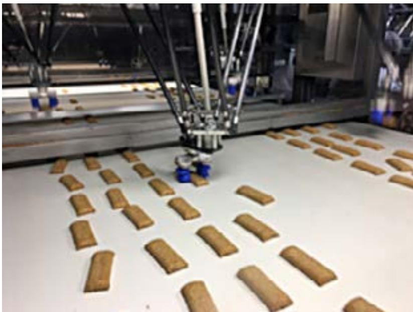
between 20 and 40 hours a week, every week, maintaining the vacuum grippers on the cereal bar packing line, all of which was virtually eliminated by the move to food-grade *mGrip* robotic tooling.
