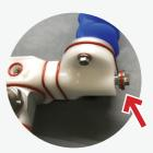
**Note:** Use the Tie Rod and spacer chart (located on the right panel of this guide) to identify which tie rod is best for your gripper. We recommend Anti-Seize gel onto the Tie Rod before M4 Hex Nut is installed.
