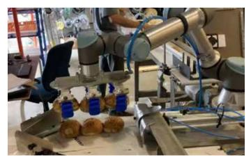
As part of the final robotic bread packaging work cell, loaves travel down a conveyor to a robotic pick station. Once there are enough loaves on the conveyor to fill one layer of a bread bag, the bread blocks a photoeye, triggering the robot into an action. A Universal Robots UR10 collaborative robot (cobot) sporting a six-finger Soft Robotics *m*Grip robotic gripper grabs the loaves in the accumulator and carries them to
