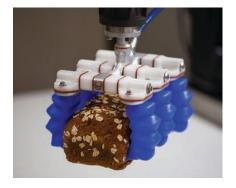
Special grippers, like this one from Soft Robotics, enable robots to handle delicate products such as baked goods.
